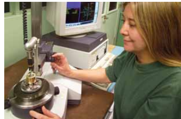
A Bracalente employee is using a Formtester, model Formscan 6100 supplied by Mahr Federal, in order to test for roundness.
